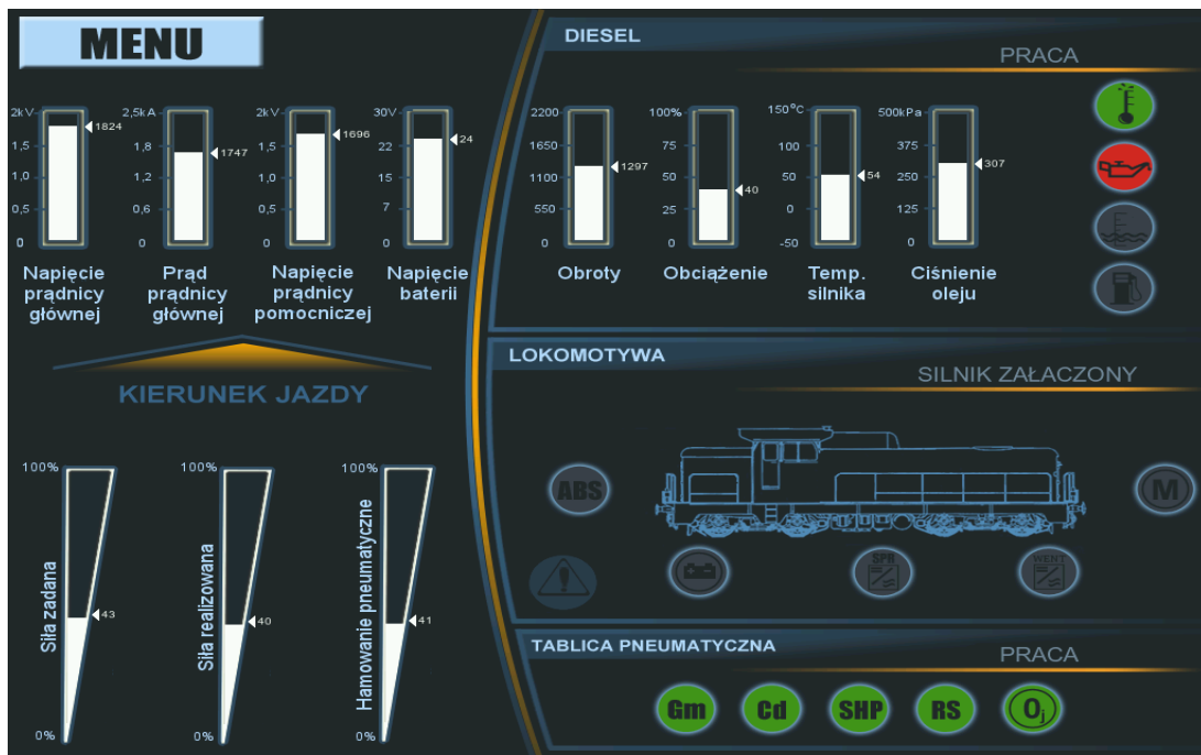
Main screen on the driver's control panel
