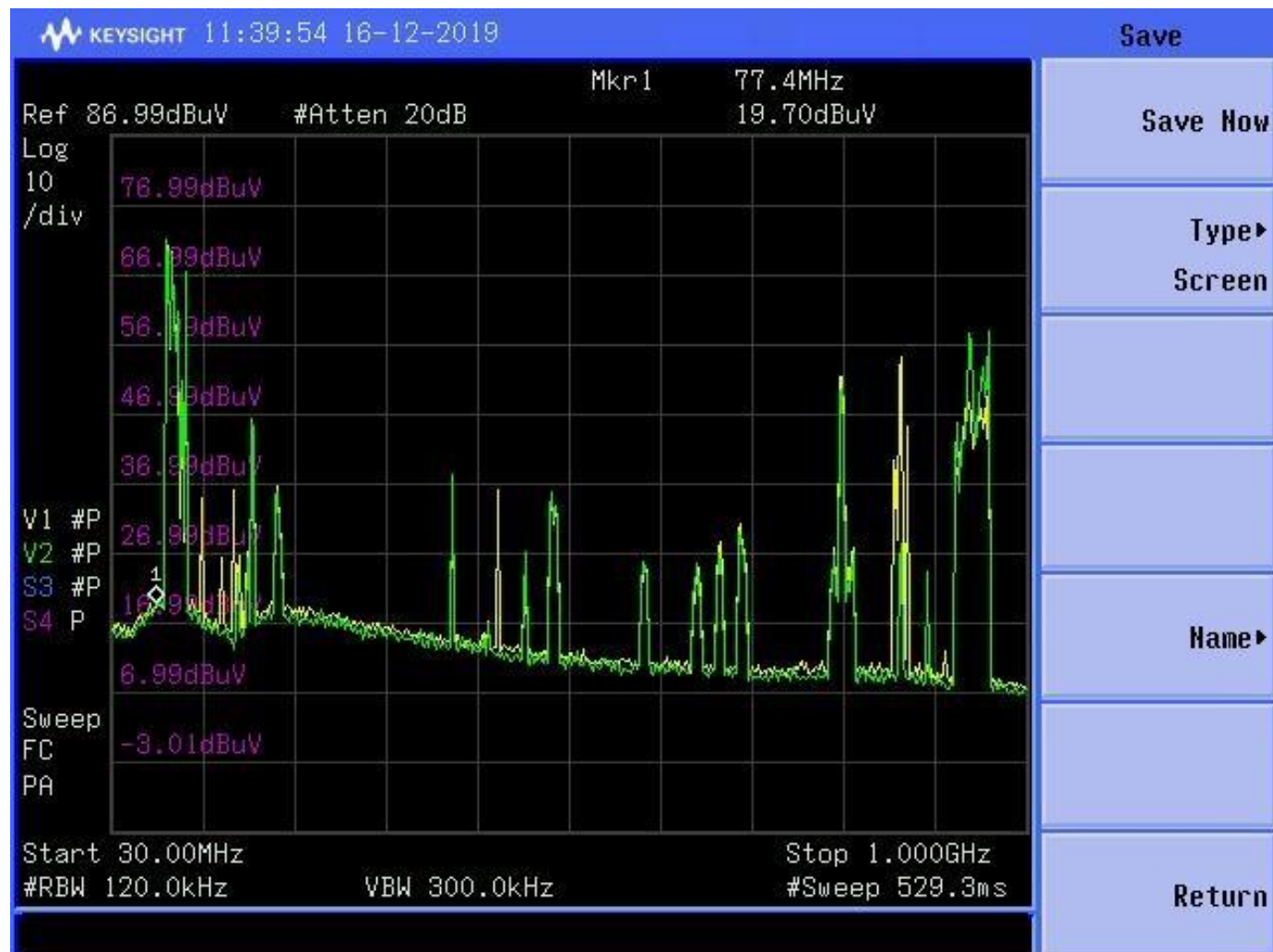
Figure 3 Radiated interference (electric field), horizontal antenna polarisation, tram in motion
