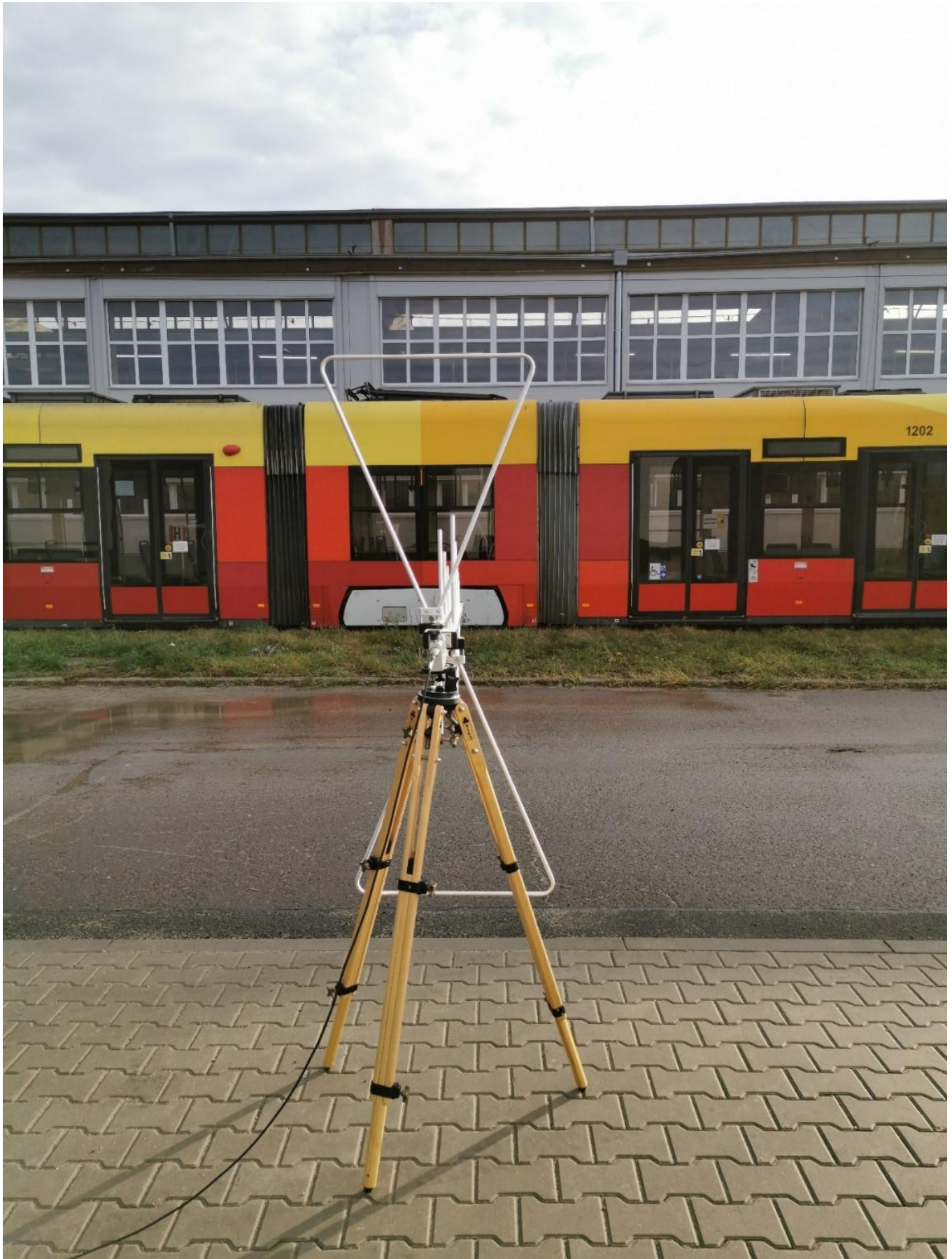
Figure 2 Electric field emission test in the 30 Mhz – 1 GHz range
