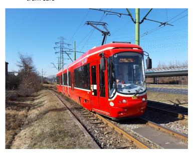
systems, replacement of the cabin and exterior lights, replacement of the door panels complete with operating drives and wheelchair access platforms, installation of all new, dark-tint window glass, repair and paint refinishing of the car bodies, installation of new passenger seats and cabin trim, installation of new cooling and heating units for the driver's cab and the passenger section, and replacement of the driver's cab rear wall, complete with a sliding door.
